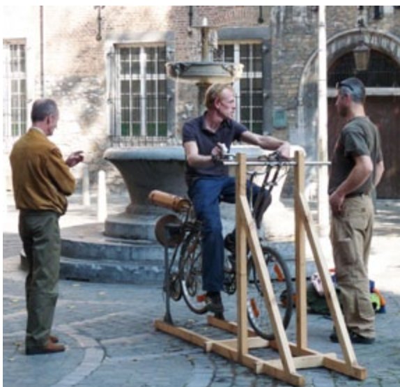
Created in 2008, this Cyclophone experiments with the principle of the hurdy-gurdy. The bicycle drive rotates a wooden wheel rubbing a drone string. The movements of the handle bar rotate the instrument, changing the rubbed string and giving the possibility to play the instrument.
